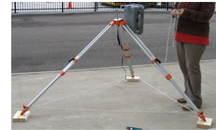
Figure 14. Active tripod setup with rope and wooden footings
