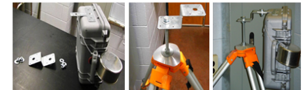
Figure 15. Mounting bracket hardware and assembly process for tripod setup
